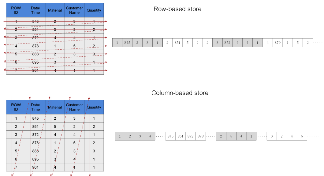
Figure 2-1 Differences between row storage and column storage
